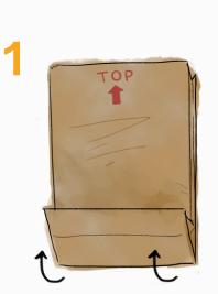
At the closed end of the bag, fold the loose flap flat against the bag's bottom
